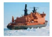
50 Years of Victory is a nuclear-powered polar-class icebreaker and the newest Arktika class icebreaker to be commissioned by the operator. She took 20 years to complete and is the largest fitted for passenger travel to the North Pole. The ship sails from her home port of Murmansk, Russia and has a steel ice belt five meters (18 feet) wide which enables her to crush through ice up to 2.5 meters (more than nine feet) thick.
